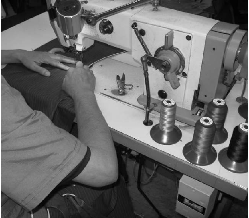
4.8 Individual sources of light on sewing machine.
